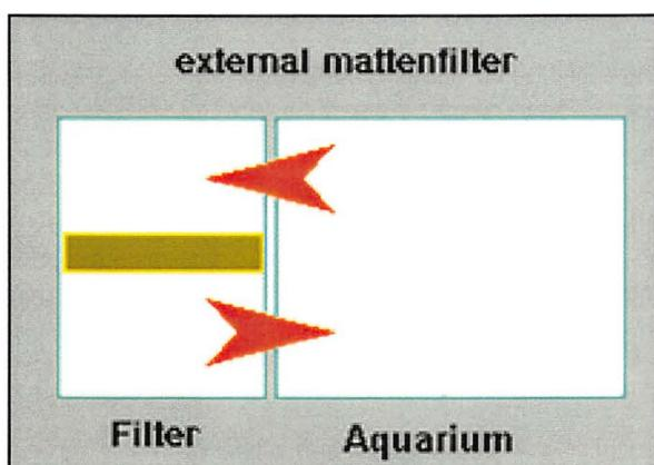
Other aquarists have moved the Mattenfilter out of the tank, into a second tank, i.e. a sump. If the balance between the size of the combined tanks, the flow rate and amount of water filtered is preserved, there really is no argument against this sort of setup. With some DIY it could even be possible to hide a sump setup underneath the tank.
