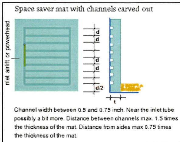
My smallest tanks are no bigger than 5 liters. These are photo tanks. I have used a construction there whereby the channels for transporting the water are carved out of the back of the foam, rather than leaving 2 cm between mat and glass.
