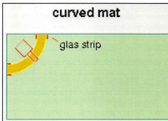
The radius should be calculated to have the required surface. The actual curve should not be too small, because the inside of the mat is compressed somewhat and will slow down the water flow a little. How far you can go depends on the actual type of foam used and its thickness.
