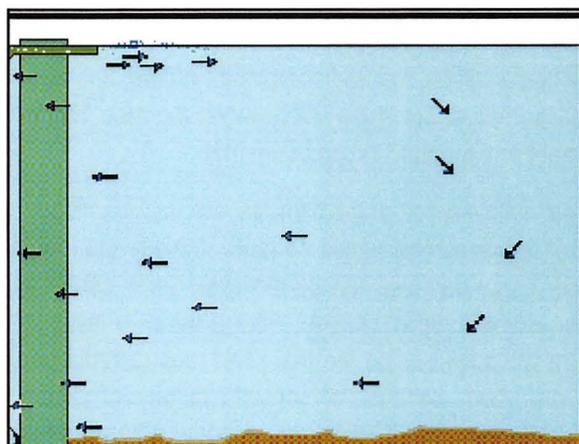
Drawing 2 shows a setup powered by an air pump. The air lift sits behind the mat. The exit tube sits in a carved out slit at the top of the mat and sticks out 5 cm to ensure that small fish will not crawl through. Some species seem to like this. These animals almost seem hypnotized by the current and are drawn into it.
